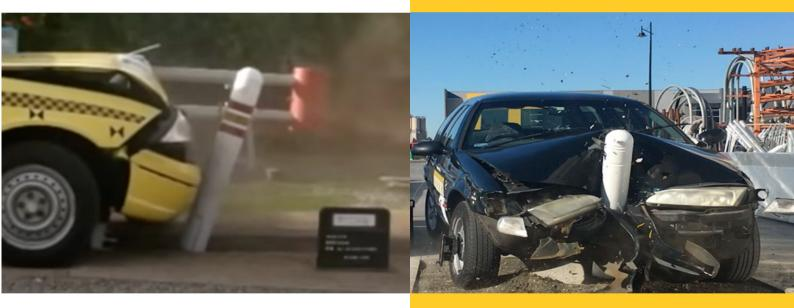
The EAB is classed as a discrete crash cushion, tested to AS/NZS 3845:1999 Table 5.3.3 (3). The EAB has a compliance sticker featured prominently to identify the standard to which the EAB complies.
